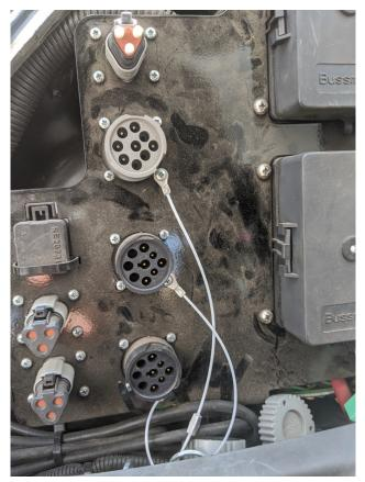
The CAT-JD Bridge adapter harness has the 2\* 4pin deutsch connectors, a 12-pin deutsch connector, and optionally a 9-pin diagnostic connector. The 12-pin deutsch goes to the CAT-JD Bridge.
