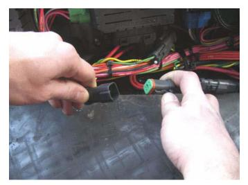
For older CAT A,B or even without letter machines, at times the iso steering is not an option. AgraGPS also has a diagnostic port adapter for these machines.
